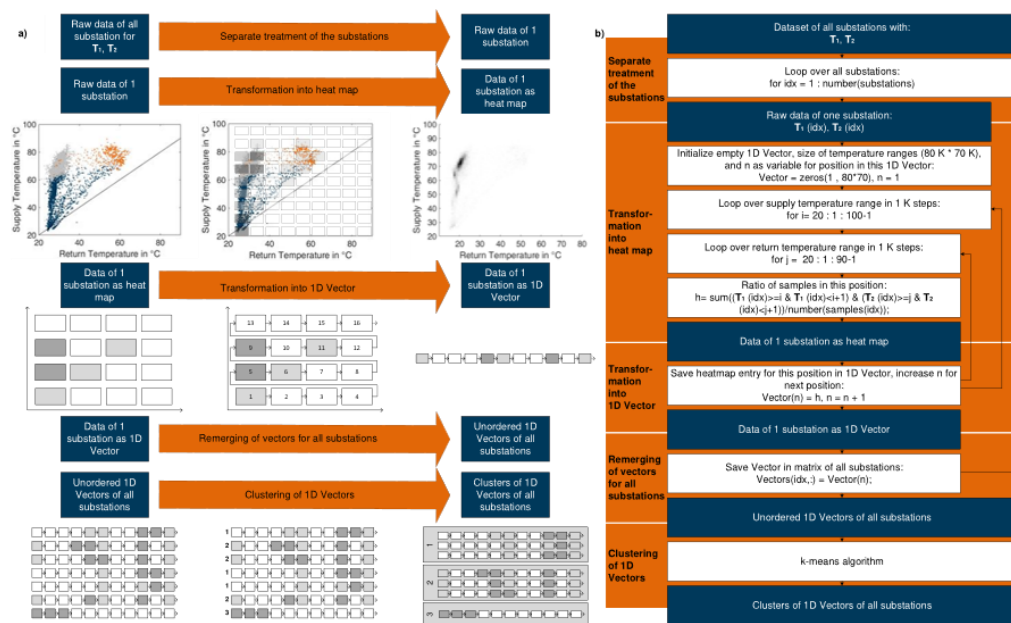
Figure S3 a) Visualization of processing steps for data pre-preparation and clustering with b) flow chart. The processing steps in orange and the data in dark blue in a) are mirrored by the flow chart in b).
